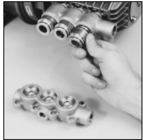
Removal of Adapter from Inlet Manifold
