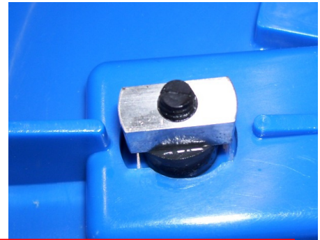
Retaining Nut Aligned for Inner Shell Removal
