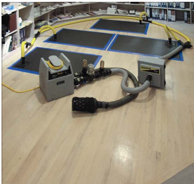
HP60, Silencer, Interceptor HEPA drying hardwood Floor with multi Port Panels
