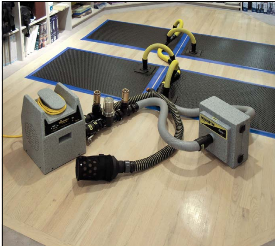
Vacuum drying and the use of HEPA Filtering systems, allows homes and businesses to be used during a dryout. (Large Single Port Panels shown)
