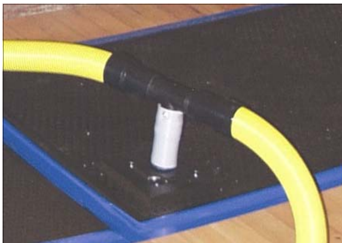
Hoseline connects to Panel T's on the Multi and Single Port Panels
