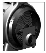
other duct attachment device or block off any other part of the inlet on the AirWolf. Doing so may reduce cooling airflow across the motor of the AirWolf, and may cause an imbalanced airflow through the Dehumidifier. This may decrease performance and cause damage to the AirWolf and the Dehumidifier.
